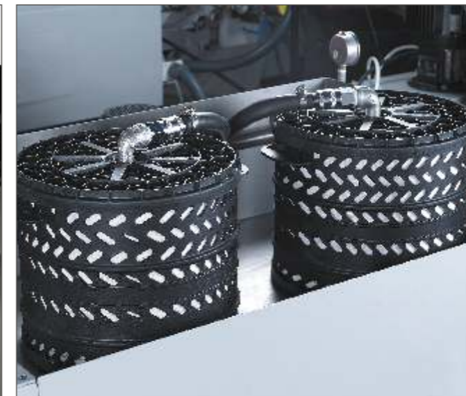
Large surface area paper filter specially designed by MANN, Germany
